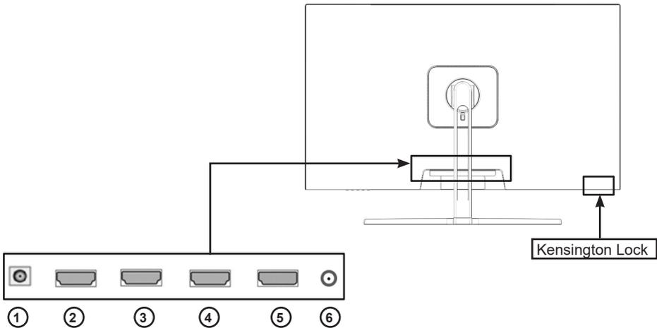
**1/ Power plug:** Connect the power adapter before use.
