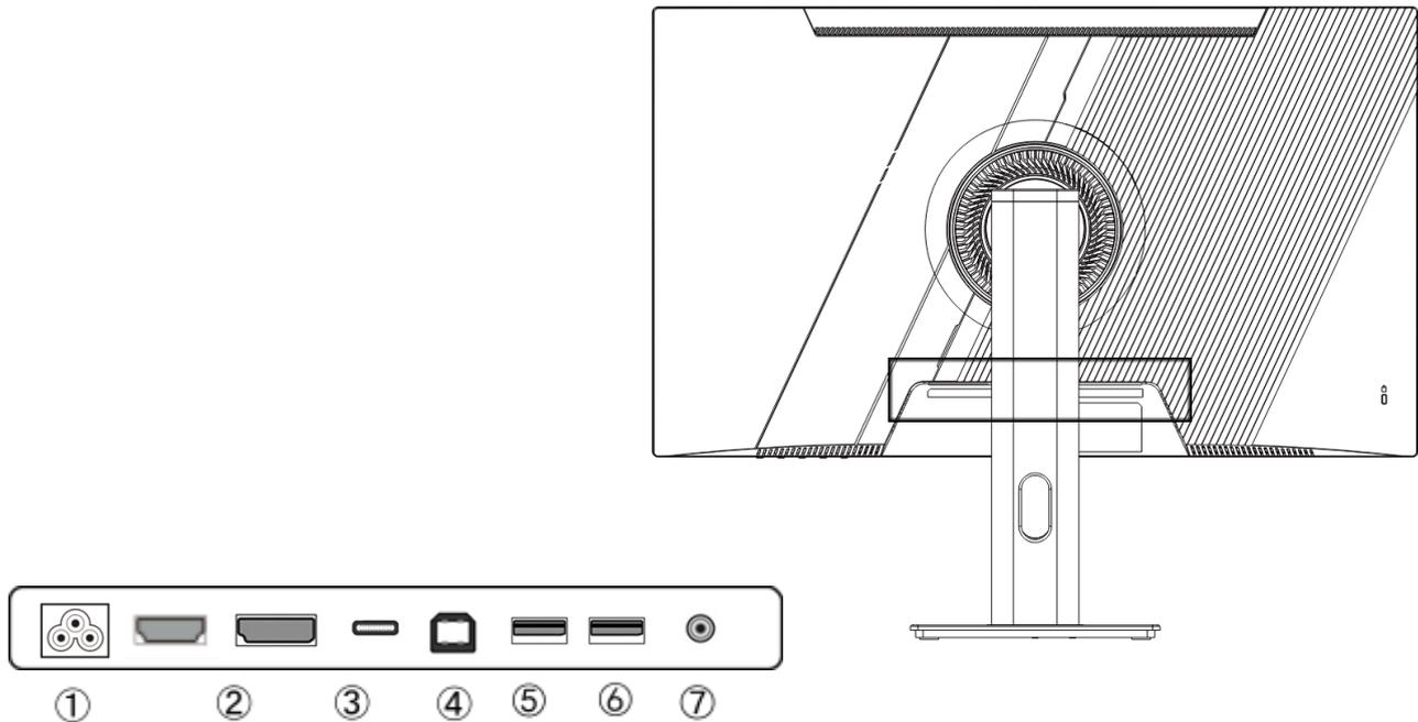
**1: Power supply:** Used when connecting the power cable.
