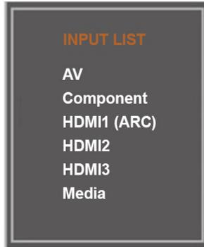
Use the ▲/▼ buttons on the remote control or the "Input Switching" button to navigate and use the "Enter / Ok" button to confirm. Press the "Return ←" button to exit the input switching screen.
