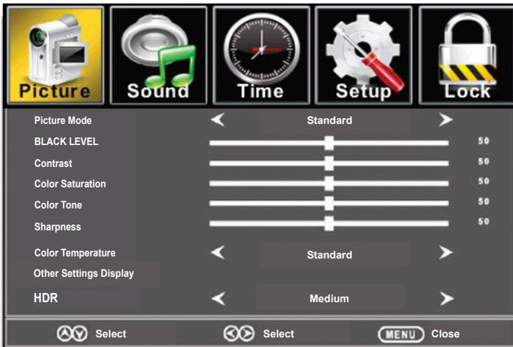
Use the left and right navigation buttons on the remote control to move between items, and the up and down navigation buttons to select menu options. To return from menu content to menu items, press the "Menu" button. Press the "Return ←" button to exit the menu screen.
